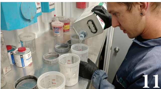
Fig. 8 - On this car we went with Spies Hecker paint. With their waterborne line of basecoats and quality clear. Fig. 9 - Mixing of the basecoat and reducer need to be right with waterborne basecoats so flash times and coverage is good and timely. So take your time and make sure your mixers are right for your application. Fig. 10 - Brian is adding activator to the base coat for the two tone. Spies recommends adding the activator to the first color to go down for proper adhesion and so your tape does not pull off your first color. Fig. 11 - Now mixing the final piece of the puzzle, clear. When mixing clear make sure your hardener is right for the temperature. The slower or the hotter temperature the hardener the longer your clear will flow and lay out smooth.
