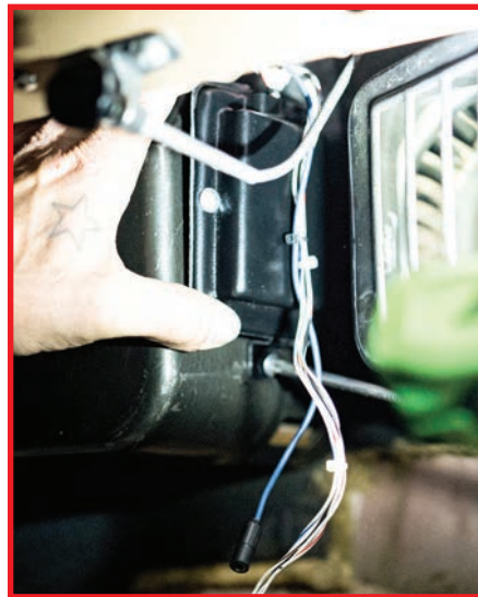
Rather than use a hidden SureFit unit, we opted for a classic styled Vintage Air under-dash universal A/C kit, keeping the "dealer-installed" look of the fifties alive and well with modern technology!
