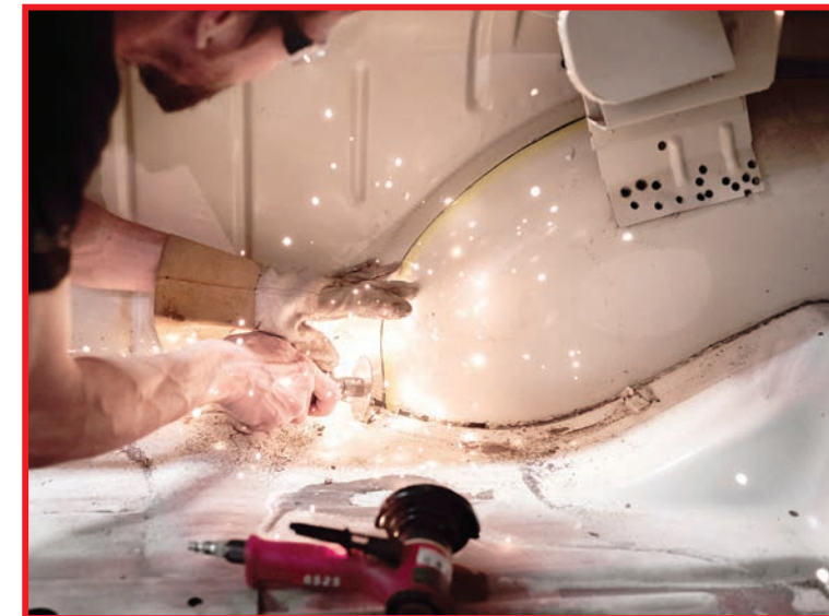
Above Left: Master builder Brian Graber cuts away the factory wheeltubs to make room for the big Billet Specialties hoops and Nitto 315/40 rubber. Above Right: The finished product: A factory appearing wheeltub, and the trunk sprayed in Woody's signature grey to match the engine bay.
