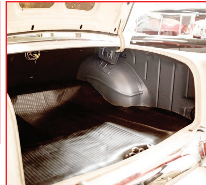
Above Left: Master builder Brian Graber cuts away the factory wheeltubs to make room for the big Billet Specialties hoops and Nitto 315/40 rubber. Above Right: The finished product: A factory appearing wheeltub, and the trunk sprayed in Woody's signature grey to match the engine bay.
