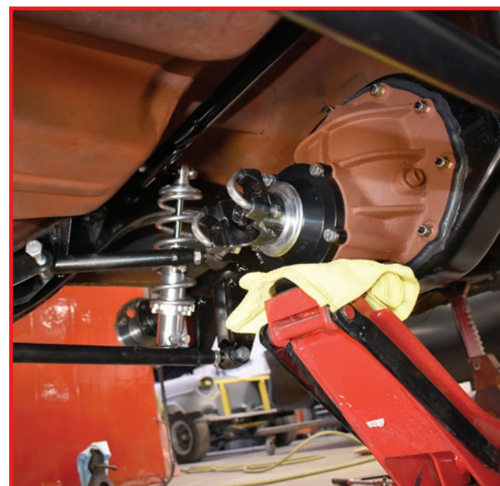
Small and weak out, big and strong in! The John's 9" replacing the factory rear will not only be light-years stronger, but leak free and 100% reliable just the same.
