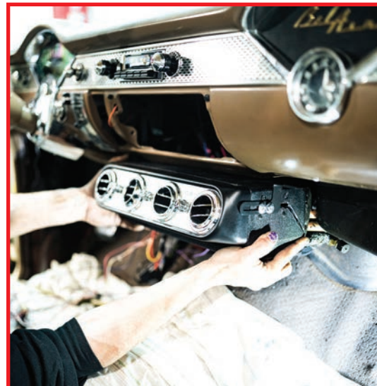
Rather than use a hidden SureFit unit, we opted for a classic styled Vintage Air under-dash universal A/C kit, keeping the "dealer-installed" look of the fifties alive and well with modern technology!
