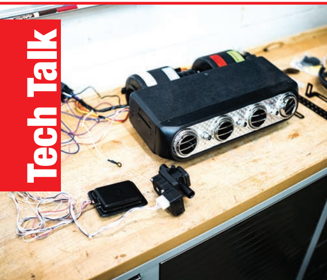
Rather than use a hidden SureFit unit, we opted for a classic styled Vintage Air under-dash universal A/C kit, keeping the "dealer-installed" look of the fifties alive and well with modern technology!
