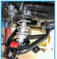
With the coilover in place, you can begin re-installing the spindle, bottom side first, then swing the upper control arm down to it.
