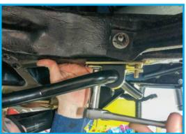
With your holes drilled, slip the u-bolts up into the frame and down through your holes, and jack the sway bar back up to meet them. Torque them down using the provided lock nuts, and tighten down your endlinks.
