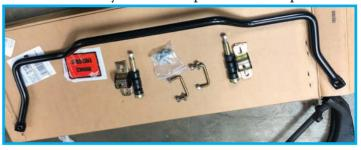
The final piece of the puzzle lies in the 7/8" front sway bar kit. This beefy kit takes out excess body roll, again without affecting ride quality. Note the kit includes 90\* angle brackets for control arm mounts. These mounts will not be used here, as our control arms already have sway bar mounting points.
