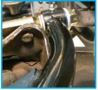
The Viking coilovers use 3/8" mounting provided hardware, where the control arms are made to accept factory 5/16" shock bolts. Rather than step up washers
