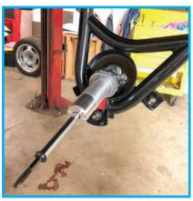
With everything greased, and your lock/height rings installed, go ahead and bolt the coilover to the control arm. Make sure to keep everything centered between mounting points to prevent binding.
