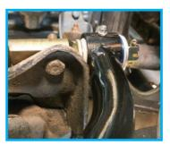
with some, all, upper control arm stands, the large diameter of the control arm tubes These arms come with will make contact in the area shown. Test fitting the upper arm before Vol. 4 Issue 7's "Front and installing the rest of the suspension will indicate over the full benefit of if any modification is required.
