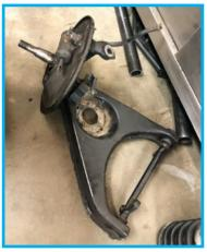
With the spring out of the way, and the spindle hanging, the control arms are next to go. You'll re-use your hardware for both upper and lower arms if it's in good shape. If not, use grade 8 bolts from the local hardware to replace. Keep track of your alignment shims for your uppers as well, it'll be a good starting point.
