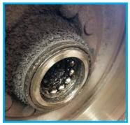
"Bearing" down! These ball bearings are one of the biggest weak points in any tri-five that sees extended amounts of use. Modern taper bearings are the key for reliability on a car that'll see highway speeds, including this one.
