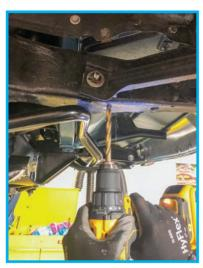
With the sway bar still dropped, go ahead and drill these holes using a 3/8" or slightly larger bit.
