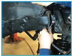
The brake hose will need to be unhooked. Since this car will be getting discs, this one will be hitting the trash!
