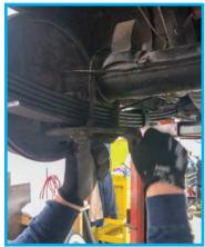
Now, you can re-install the spring plates and your u-bolts Make sure the shock mounting stud is free of rust and clean, if your leaf spring plates have any excess corrosion on the stud, use CPP-5557LSP to replace. A thin coating of grease on the stud will aid installation in the shocks.
