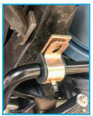
With the bushings and retainer slipped into place, jack the sway bar up until it makes contact with the frame. Go ahead and mark only the front mounting holes. Then, drop the sway bar out of the way, and use the u-bolts to measure out and mark the rear holes.
