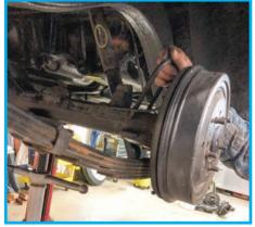
With the shock plates out of the way, remove the u-bolts. If yours are in rough shape, have the guys at Woody's add WHR-80016, quantity of 4 to your kit.
