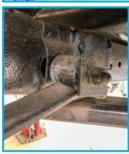
Once the spring is loose from the front pocket, swing it down and unbolt the rear shackle retainer. Once the retainer is off, you should be able to wiggle the spring free from the shackle itself. If you're With the u-bolts, shocks, and plates out of the way, go ahead and remove the front eyelet bolt through the access hole in the frame. You may need to give it a whack or two with a drift pin, as they may have been in there for 60+ years. A set of extra hands really comes in handy.
