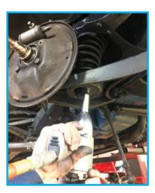
....bottom comes next. With the lower shock bolts removed, it'll simply slip through the lower control arm. Again, these will not be reused.
