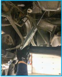
traction on launch for the horsepower enthusiasts. Slide the shock onto the spring plate first, as this may take some wiggling, and you don't want to fight the upper bushings. Install the nut, and install the lower half of the bushing onto the shock rod, and extend the shock rod through the trunk or shock bar.
