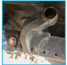
With the shackle out clean up the inside of the perch on the frame. A generous helping of grease here will ease installation and yield quiet operation. Remember, the shackle is supposed to move!
