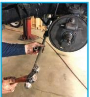
You'll need to remove the tie rods from the steering arms. Typically a whack or two to the steering
