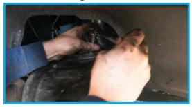
At this point, we'll go ahead the remove the shock. I tend to always do the top first, as a little tension on the setup may or may not let you get the top nut off without holding the rod.
