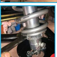
With the spindle in place, go ahead and torque the ball joints and install cotter pins, as well as torque the top shock bolt. And there you have it, a fully assembled new front suspension! If you were reusing your steering, now would be the time to reinstall those parts. We'll be covering that in coming months.
