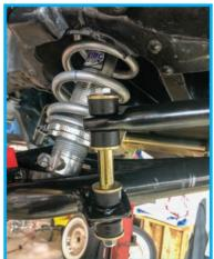
Carefully lift the sway bar into place. You can use a floor jack to support to middle section of the sway bar, as you'll need to make some marks pertaining to mounting coming soon. Go ahead and bolt the sway bar end links all the way on as shown, leaving them only hand tight.
