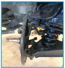
Some cars may start separating here with no coercion, that'll make life easy. If not, a whack or two to the spindle should set it free, the tension from the spring will help.. The nut in place will keep it from coming all the way apart.
