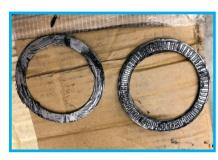
The Viking coilovers also come with a roller bearing for ease of height adjustment. A coating of grease here will keep things moving as they should for years to come.
