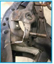
Clearance can accomplished with some heat and a hammer, or simply trimming a small amount away with a grinder. Again, how much will vary per car. We only needed a very small amount with this one.
