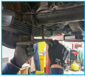
Now we move on to the back. The Del Ray received newer poly button springs at some point, but at stock ride height. This one will certainly reap the benefits and improved handling of a lower center of gravity without sacrificing ride quality, not to mention a killer stance. Support the rear end, and unbolt the factory shocks and lower shock plates.
