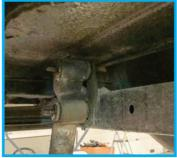
replacing the shackle bushings like we are, swing the shackle above the frame, and slide it off. This may take some help from a pry bar, depending how long they've been in place.
