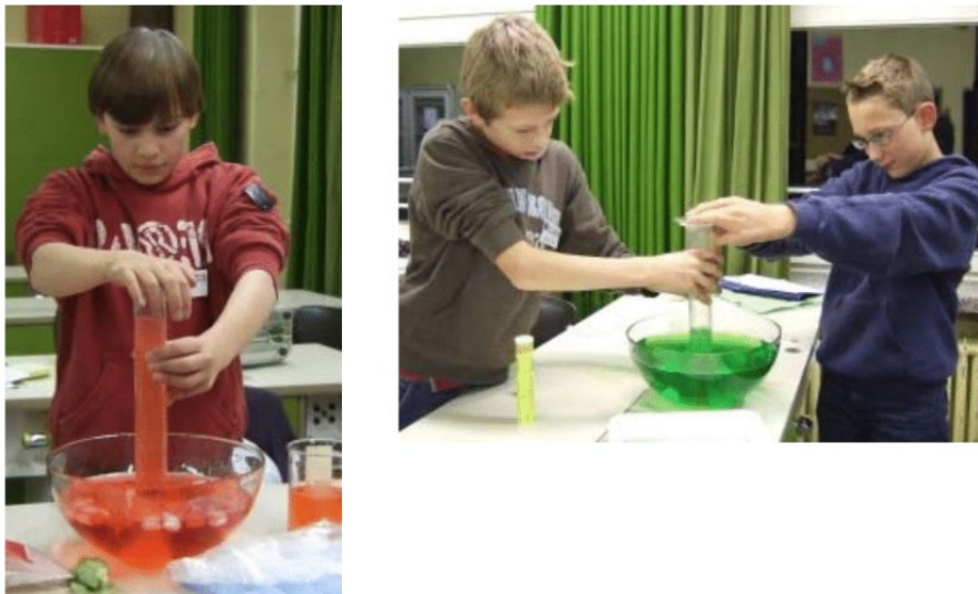
Fig. 3 The air space formed at the top of the cylinder is smaller when cold water is used (left photo, note the ice cubes). When the water is warm a bigger air space is formed (above)
