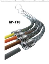
The MAXIS® grips pulling heads are a dual lock pulling system that uses both a cam lock head and a double braided wire to quickly secure cable to rope without the fear of losing a conductor. These pulling heads provide increased efficiency with 2 minute head preparation.
