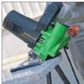
Stepless mitre adjustments up to 45° – without tools
