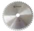
Carbide-Tipped Blade for General Use, 7" dia. (180MM) P/N 9 2503 0120 36T, to cut metal, plastics and wood.
