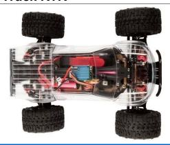
EMB-MT is with big tires to cover all terrain and strong bumper to bash, with High power and efficient 4 pole 2838 brushless motor, All aluminum gear differential, 35A programmable ESC, Batan 2.4GHz Radio System, and High rate 7.2V NiMH battery on smart charger.
