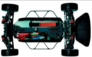
EMB-WRC is for fun control on four power wheel to slide, with High power and efficient 4 pole 2838 brushless motor, All aluminum gear differential, 35A programmable ESC, Batan 2.4GHz Radio System, and High rate 7.2V NiMH battery on smart charger.
