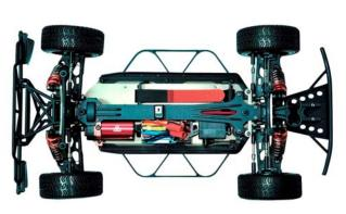
EMB-SC is for more bashing on bumper even small, with High power and efficient 4 pole 2838 brushless motor, All aluminum gear differential, 35A programmable ESC, Batan 2.4GHz Radio System, and High rate 7.2V NiMH battery on smart charger.
