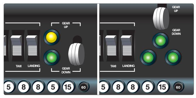
Figure 11-11. Landing gear handles and single and multiple light indictor.
