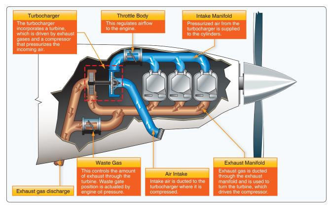
Figure 11-9. Turbocharging system.
