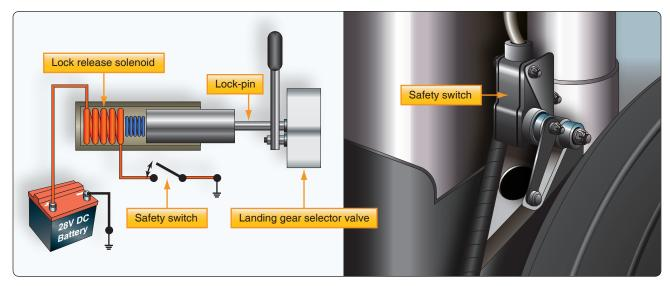
Figure 11-12. Landing gear safety switch.
