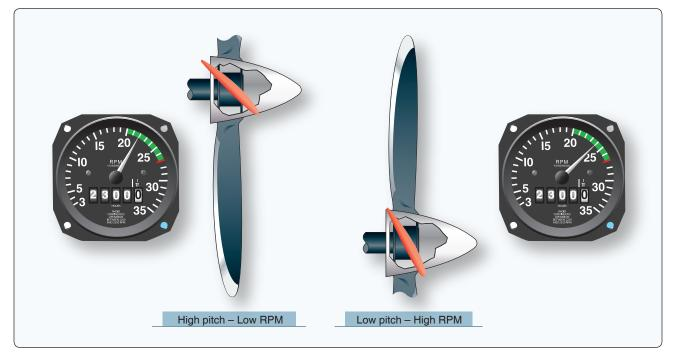
Figure 11-6. *Controllable pitch propeller pitch angles.*
