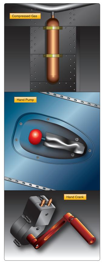
Figure 11-13. *Typical emergency gear extension systems*.
