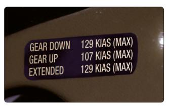
Figure 11-15. Placarded gear speeds in the cockpit.
