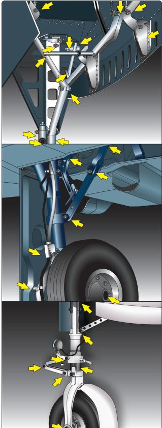
Figure 11-14. *Retractable landing gear inspection checkpoints.*
