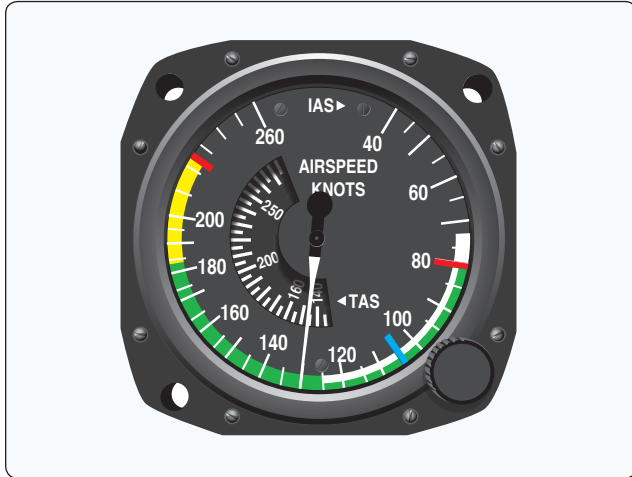
Figure 12-1. Airspeed indicator markings for a multiengine airplane.
