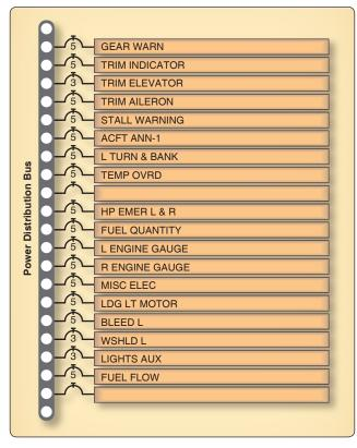
Figure 14-9. Typical individual power distribution bus.
