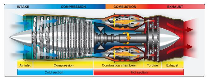
Figure 14-1. Basic components of a gas turbine engine.
