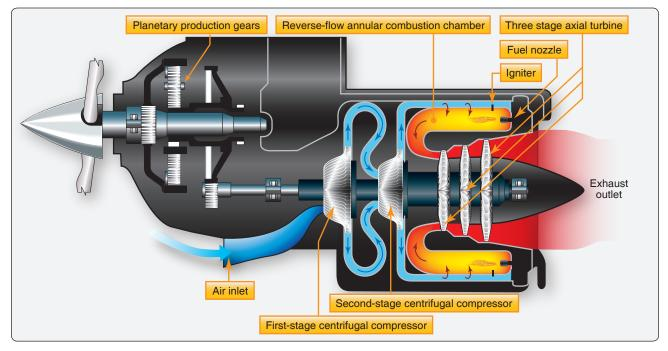
Figure 14-2. Fixed shaft turboprop engine.
