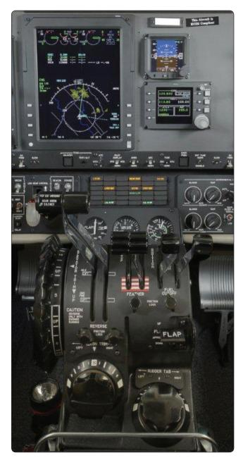
Figure 14-6. *Powerplant controls—split shaft/free turbine engine.*
