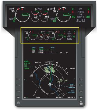
Figure 14-7. Engine instruments—split shaft/free turbine engine.
