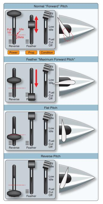
Figure 14-8. *Propeller pitch angle characteristics*.
