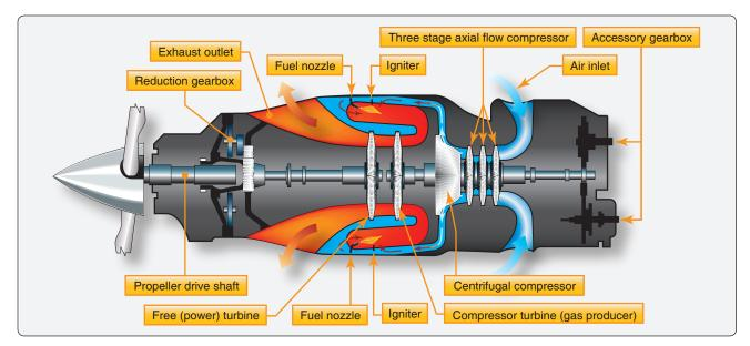
Figure 14-5. Split shaft/free turbine engine.
