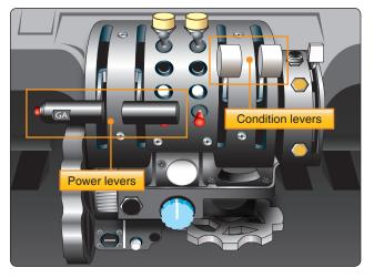
Figure 14-3. *Powerplant controls—fixed shaft turboprop engine.*
