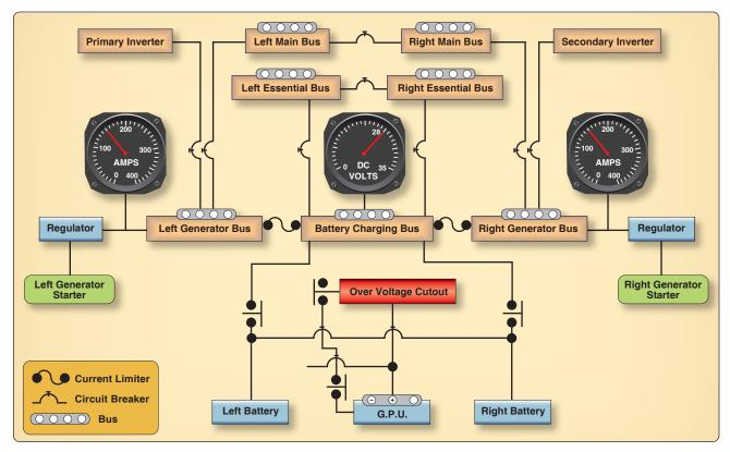
Figure 14-10. Simplified schematic of turboprop airplane electrical system.
