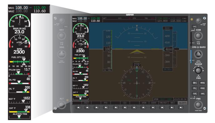
Figure 14-4. Powerplant instrumentation—fixed shaft turboprop engine.
