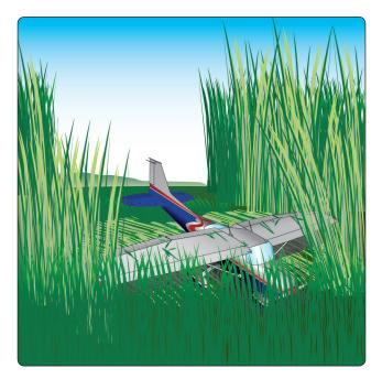
**Figure 17-1.** *Using vegetation to absorb energy.*
