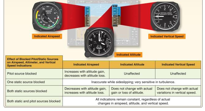
**Figure 17-10.** *Effects of blocked pitot-static sources.*
