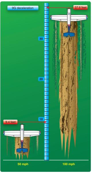
Figure 17-2. Stopping distance vs. groundspeed.
