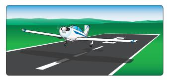
Figure 17-7. Landing with one main gear retracted.
