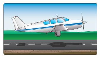
Figure 17-8. Landing with nosewheel retracted.
