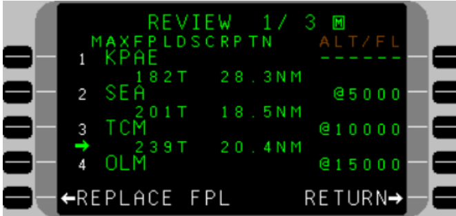
Example FMS Route REVIEW Page 1/3 Received from FPL FV2.X (SCN 1002/1102.6 and later)
