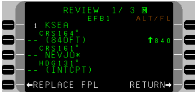
Example FMS Route REVIEW Page 1/3 Received from EFB 1 with SID Included in Flight Plan (SCN 1002/1102.6 and later)
