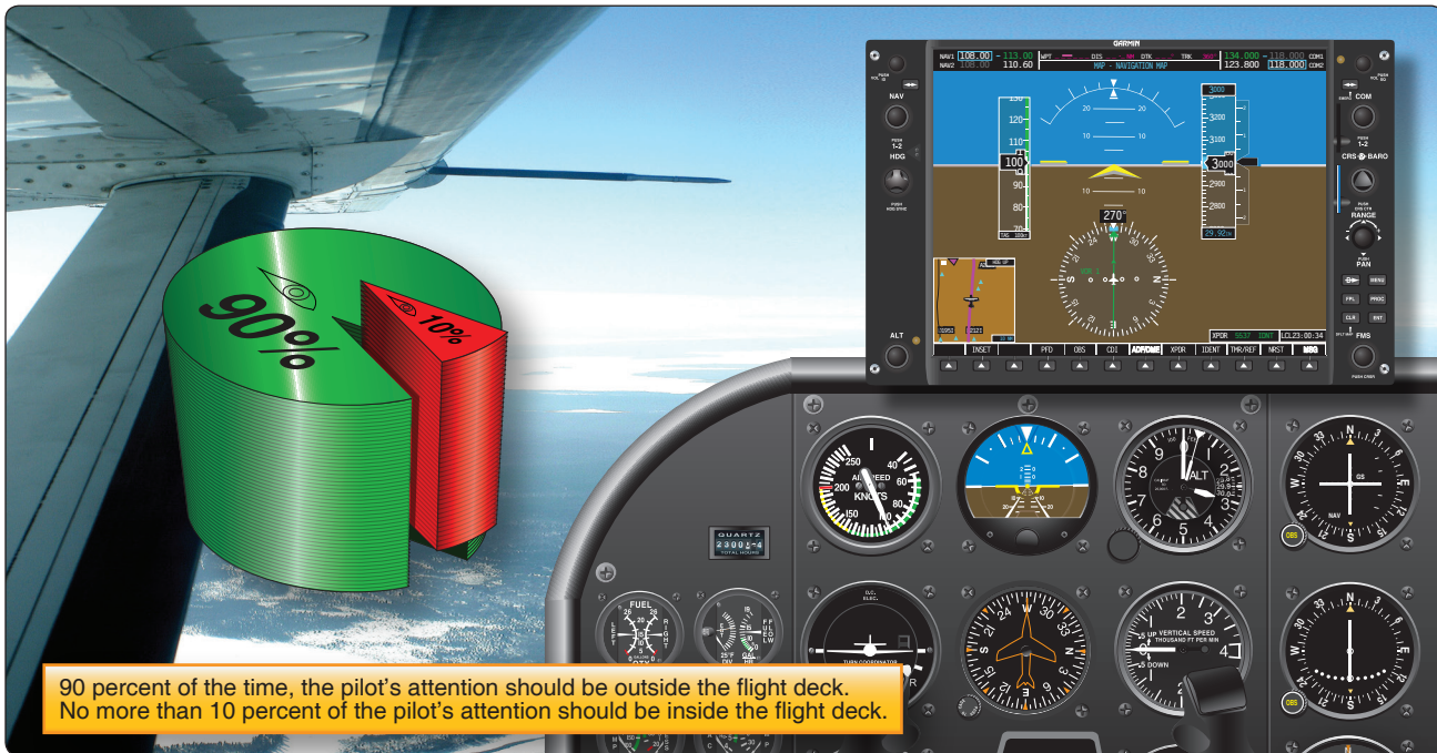
Figure 3-5. Integrated flight instruction teaches pilots to use both external and cockpit attitude references.
