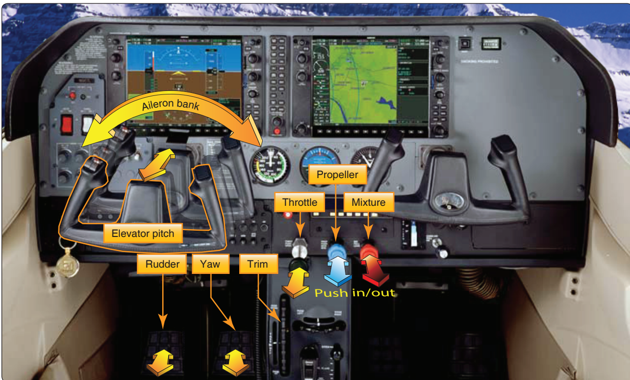
Figure 3-1. Basic flight controls and instrument panel.
