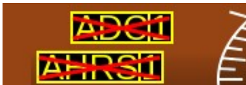
Primary Source Failed Annunciators
