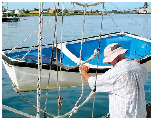
Once the two halves are mated, they switch the forward bridle legs to the bow for launching.
