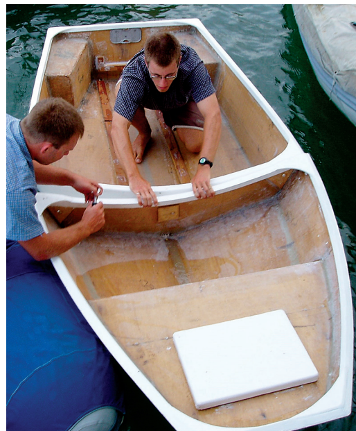
A Chameleon nesting dinghy can be assembled or disassembled with both sections in the water.
