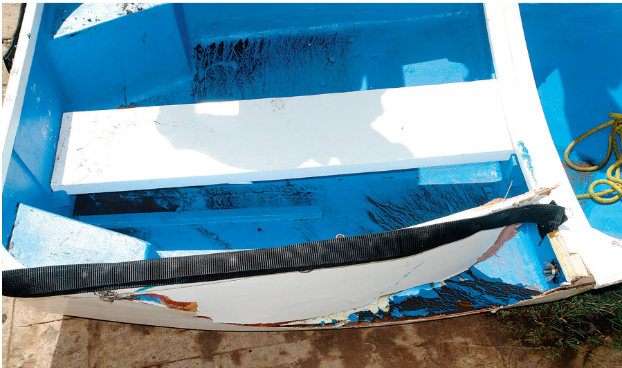
Bacio's rugged construction probably saved Philip's life when he was hit broadside by a speeding powerboat in Nuku Hiva, above. The collision stove in the starboard aft hull panel, leaving the forward half of the boat undamaged. When repairing Bacio , three photos at right, Philip and Leslie made do with the limited supplies they had on board together with what was available in their remote location. She was afloat again in a week.
