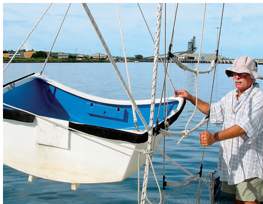
To launch Bacio , Philip and Leslie first turn her aft half upright and hoist it with a halyard.
