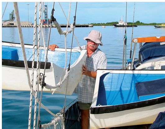
With Bacio 's stern suspended, they flip her bow half and turn it so the bulkhead faces outboard.
