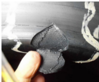
TIRE BEAD DAMAGE
