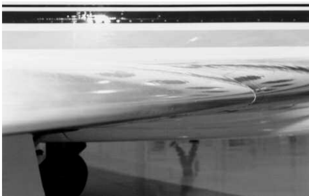
30. WING CHECK FOR FUEL LEAKS—CHECK
