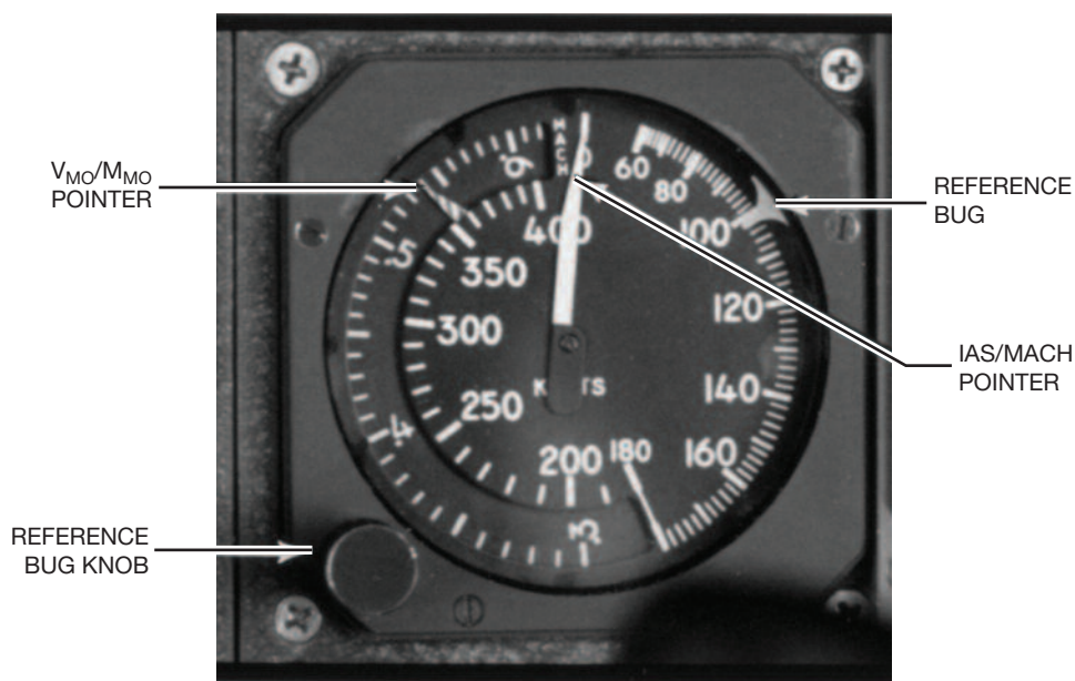
Figure 16-6. Mach-Airspeed Indicator
