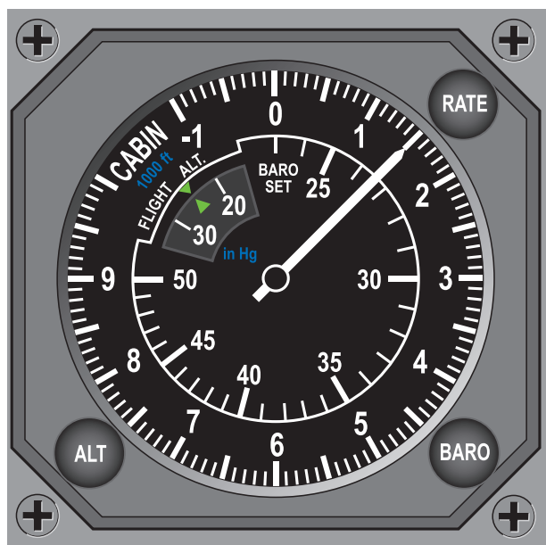
Figure 12-5. Automatic Pressure Controller
