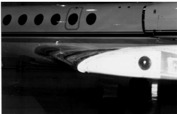
59. WING CHECK FOR FUEL LEAKS—CHECK
