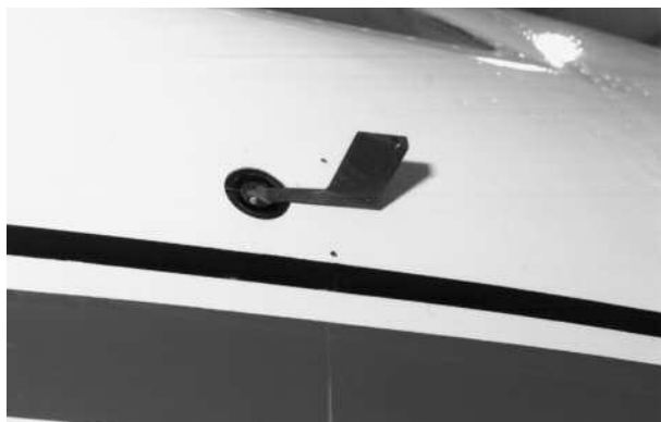
2. STALL WARNING SENSOR COVER/CONDITION —REMOVE/CHECK
