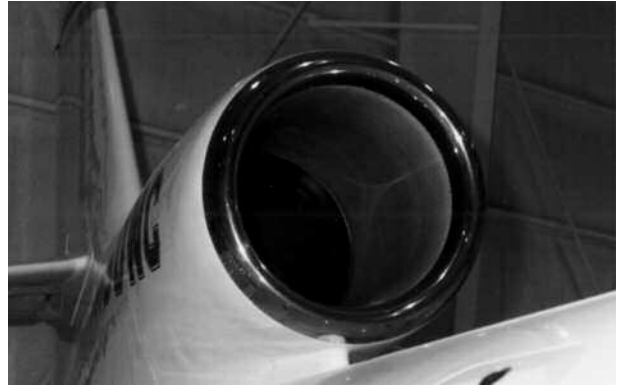
24. CENTER ENGINE AIR INTAKE COVER/CONDITION —REMOVE/CHECK
