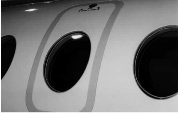
65. LH EMERGENCY EXIT—CHECK
