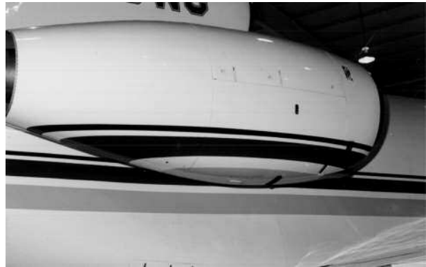
37a. RIGHT ENGINE NACELLE AND PYLON—CHECK
