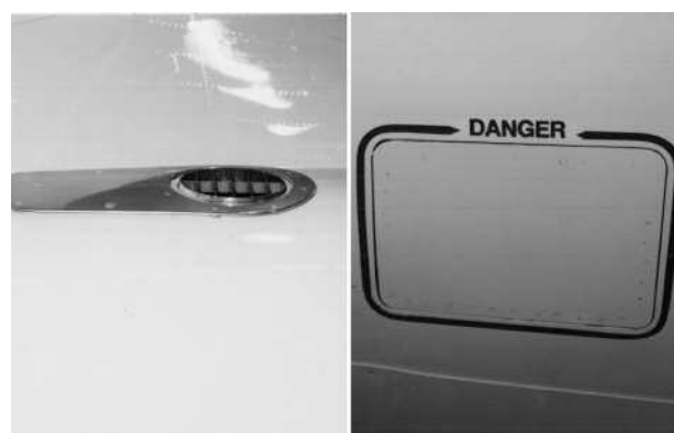
42. APU AIR INTAKE EXHAUST—CHECK
