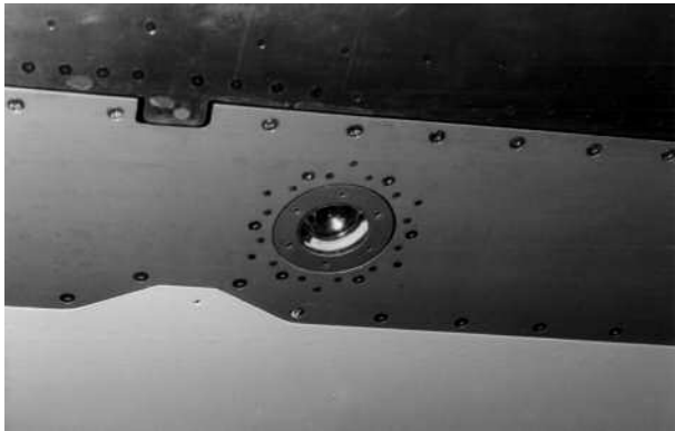
27. EMERGENCY EXIT LIGHT LEADING EDGE CONDITION—CHECK
