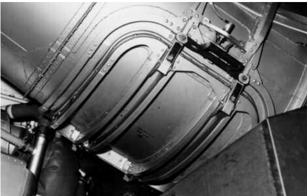
48g. REAR COMPARTMENT "S" DUCT DOOR CLOSED AND LATCHED—CHECK
