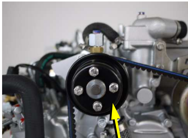
Fig. 3.3.2-4: Internal Fresh Water Cooling Pump
