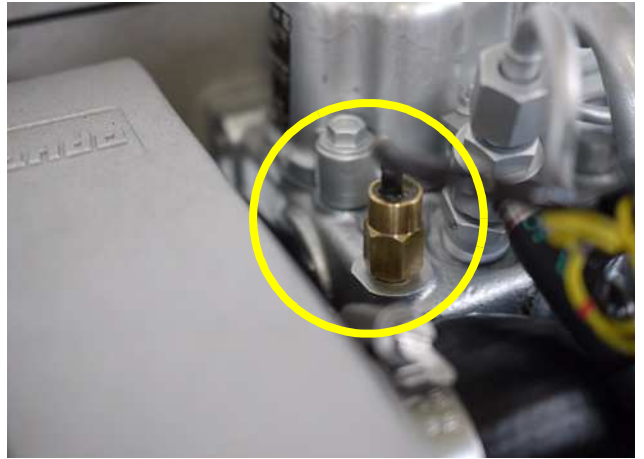
Fig. 3.3.6-1: Thermo-switch at cylinder head
