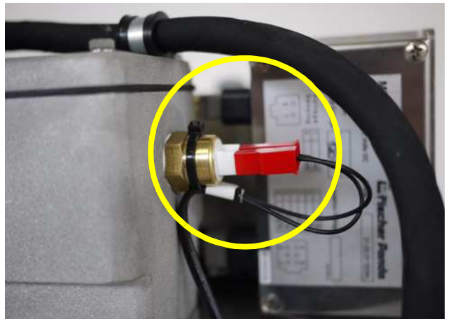
Fig. 3.3.6-2: Thermo-switch at exhaust elbow
