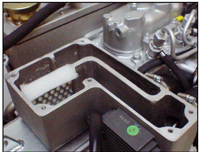
Fig. 5.4.3-2: Opened Air Suction Housing
