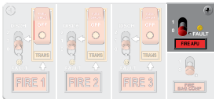
Figure EP-2. Fire Panel and Warning Lights—FIRE APU
