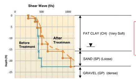
"... an average shear-wave velocity increase through the 22.6' thickness... on the order of 26% was determined.."
