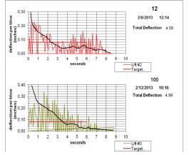
Rammer stroke deflection monitoring during actual pier construction confirmed that the design pier modulus was achieved
