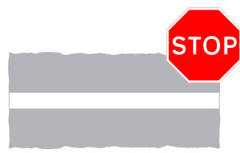
Stop line at 'Stop' sign
