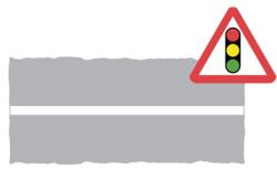
Stop line at signals
