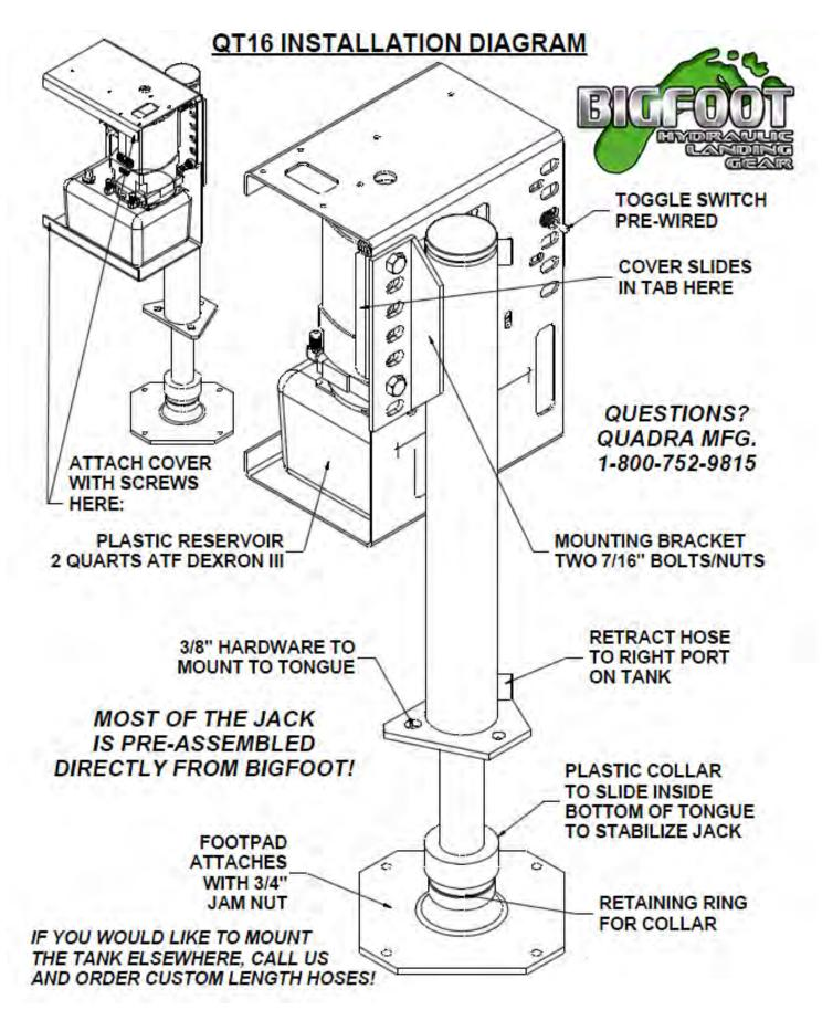
To hookup the power attach the supplied eyelet to each end of the supplied 5' battery cable. Attach one end of the cable to the positive battery terminal, place the other end to the lower solenoid post with the copper strip on the tank assembly. Auxiliary ground may be recommended, attach to a solenoid mounting stud on each solenoid and route 10 ga. cable to frame or negative terminal of battery.
