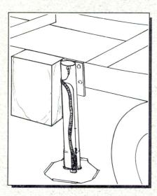
With an 85.5 square inch steel support foot, your motorhome can be leveled and stable even in loose sand or wet soils.
