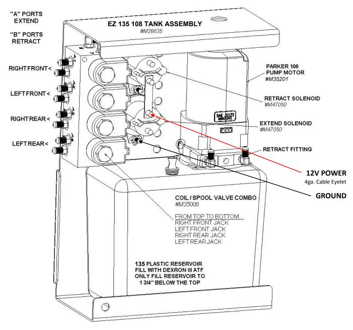
Central tank assembly is typically located near the "center" of the unit, Example: In front of rear axle on driver side frame rail (outside or between rails). Can be mounted to existing boxes, sub-frame, etc.
