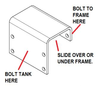
strong enough to support the weight of the assembly (7/16" hardware and lockwasher required, torque to 70 ft/lbs.).
