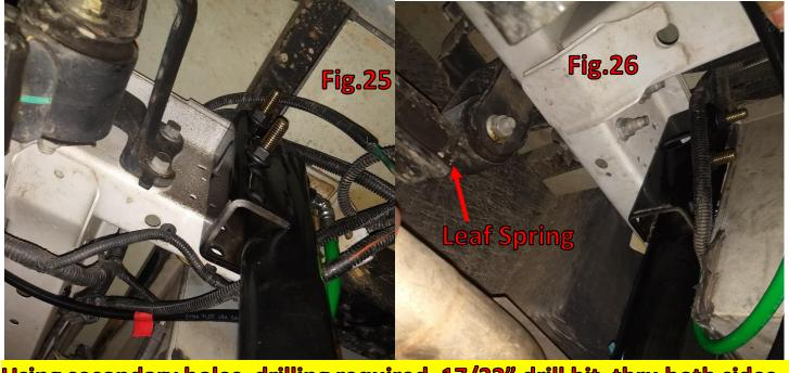
Using secondary holes, drilling required, 17/32" drill bit, thru both sides..
