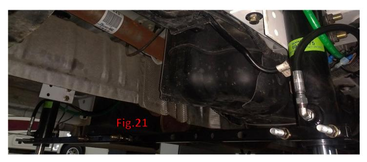
See page 14: ATTACH CROSSBRACE AFTER BOTH JACKS INSTALLED USING 9/16" DEEP SOCKET & WRENCH. SQUARE TUBE & U-BOLTS WRAP UNDER FITTING AND LIMIT SWITCH BARREL JUST ABOVE THE FOOTPAD. FIND TWO HOLES IN CENTER OF UNIVERSAL TUBES THAT LINE UP, INSTALL TWO 3/8" X 2.5" BOLTS, LEAVE ALL HARDWARE LOOSE UNTIL ALL BOLTS ARE IN PLACE, TIGHTEN UNTIL SQUARE BRACE STARTS TO CRUSH.
