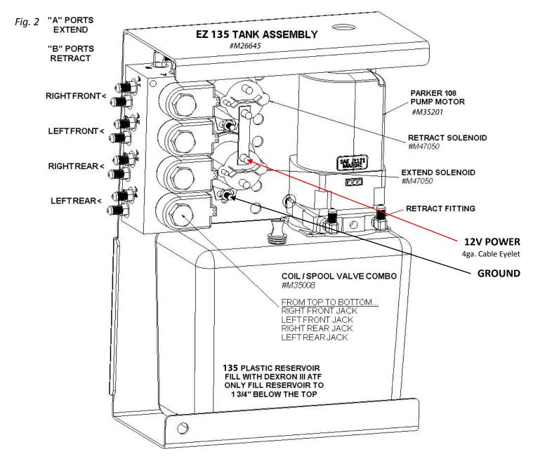
Central tank assembly is typically located near the "center" of the unit, Example: In front of rear axle on driver side frame rail (outside or between rails). Can be mounted to existing boxes, sub-frame, etc.
