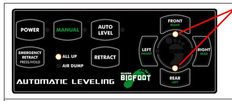
FRONT RIGHT & REAR LEFT LIGHTS FLASHING, THIS MEANS LOW VOLTAGE TO CONTROLS, PANEL INOPERABLE EXCEPT EMERGENCY RETRACT, SEE "LOW VOLTAGE CODE" ON NEXT FEW PAGES.
