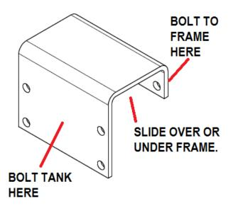
strong enough to support the weight of the assembly (7/16" hardware and lockwasher required, torque to 70 ft/lbs.).
