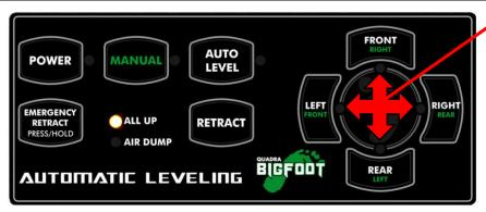
IF ONE OR MORE OF THESE LIGHTS ARE FLASHING IN ANY ORDER OTHER THAN LISTED ABOVE, NOTHING IS WRONG. THEY ARE INDICATING THE LOW POINTS OR "LEVEL STATUS" OF THE VEHICLE.
