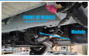
Remove the module with the two M8 self-threading bolts (set aside).
