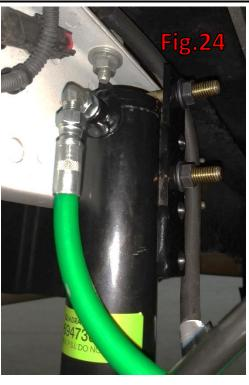
Note Fig.23, Cylinder has spacers between frame & cylinder for clearance between cylinder and plumbing near bottom of cylinder in pic.
