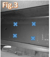
If mounting the rear cylinders directly to the outside of the frame, follow same basic procedure and mark holes in the frame though the cylinder's holes at correct height and position, drill holes and utilize at minimum four 7/16" Grade-8 bolts per cylinder and tighten to 70 ft/lbs. Make sure the supplied cross-brace is used when mounting the cylinders between the frame rails.
