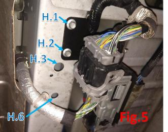
Locate "Front Nox Module" located on passenger front cylinder location under cab's passenger seat shown in Fig.5. Remove two 8mm bolts with 10mm socket (keep bolts),
