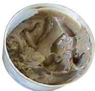
Used grease: colour turned greyish
