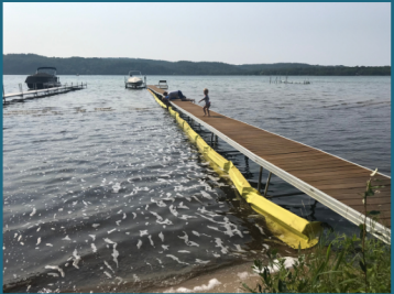
Experimental baffle along a dock shielding the larvae from a swim area.
