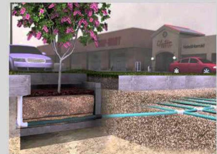
Bio-filter and storage
