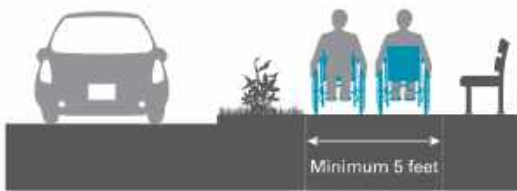
Minimum sidewalk width for ADA is 5-FT. (2020 Louisville CSDG)
