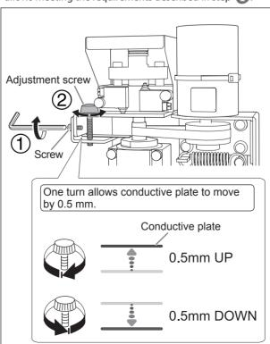
S Fix the position of the conductive plate.
