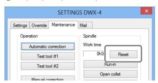
Perform running-in operation for the spindle unit.
