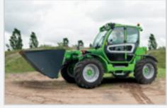
**BSS** hydropneumatic suspension of the boom (optional), which can be activated by the operator, automatically deactivates under 3 km/h to ensure maximum precision in the positioning of the loads.
