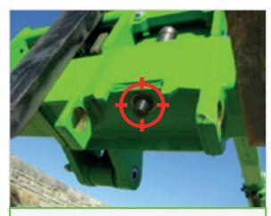
Tac-Lock: hydraulic attachment clamping system from the cab
