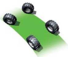
FRONT WHEEL STEERING MODE
