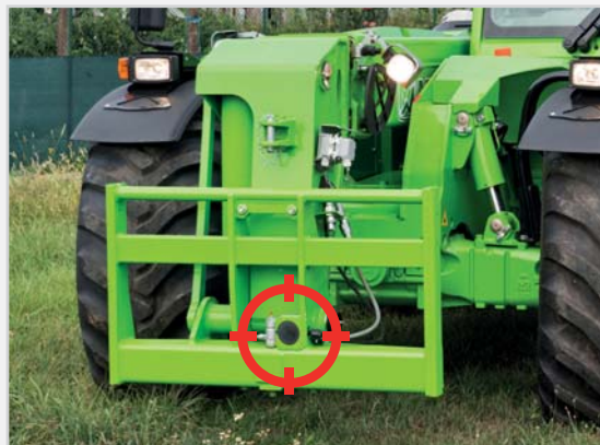
Sensor on the carriage.
