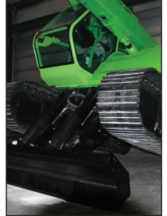
VBLADE leveling enables working on slopes up to 19° (34%)
