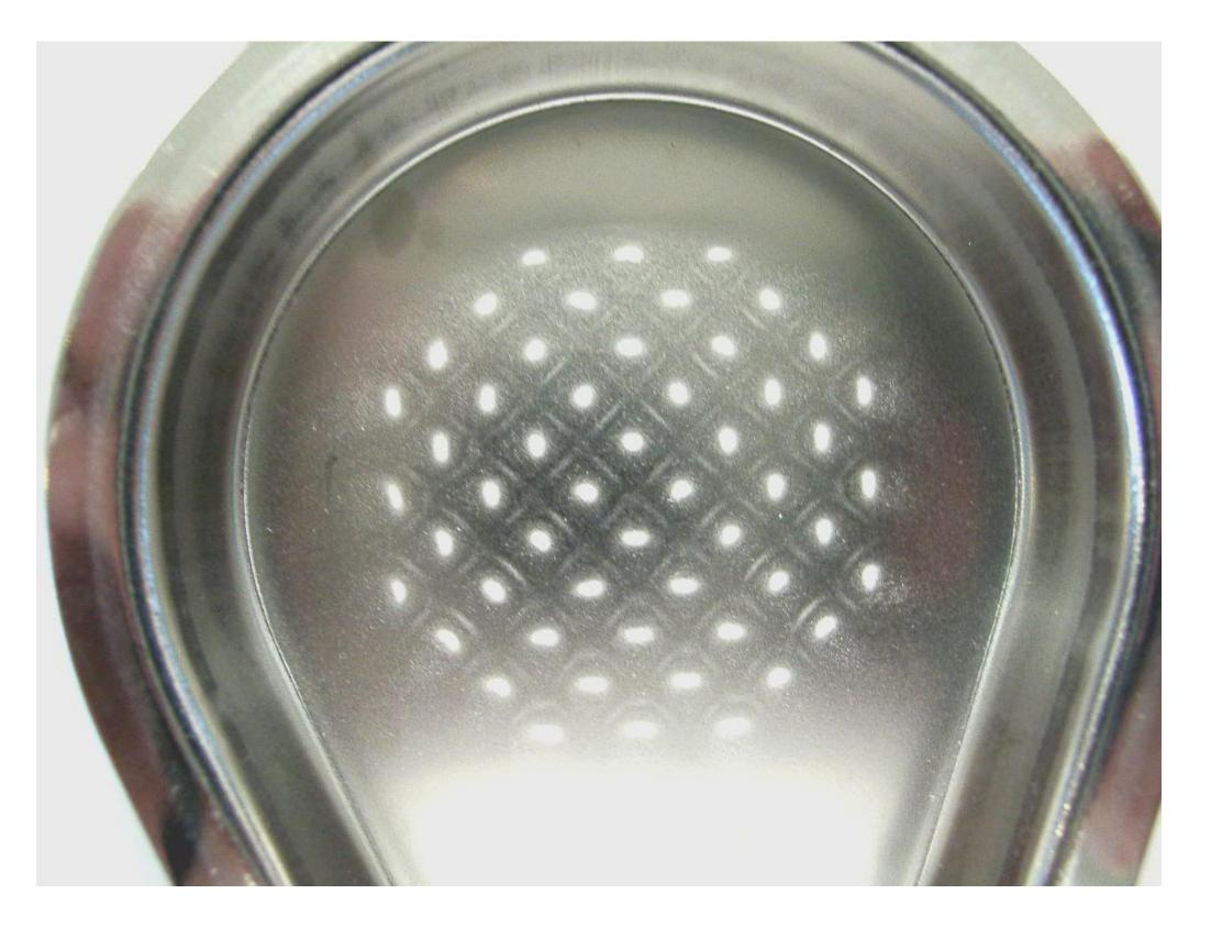
Figure 5 : Unexpected loading pattern – lines observed on plate between impaction areas
