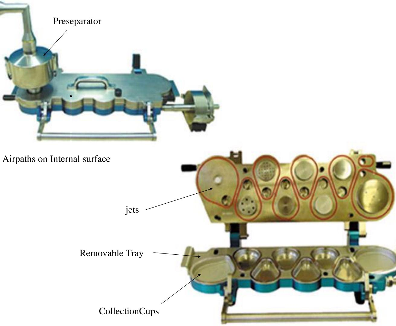
For all of the above experiments an assessment of the recovery achievable from the collection cups was made, in addition the amount of drug retained in airpaths and jets were quantified.
