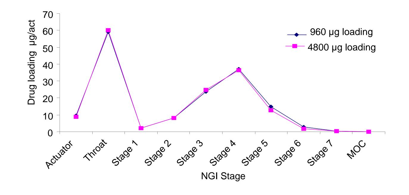
Figure 2: Effect on Impaction profile produced between high and low loading on the NGI
