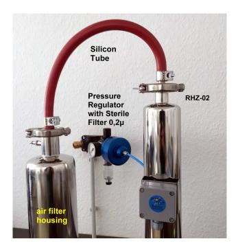
The heater must be operated with the purified compressed air, nitrogen or via a terminal sterile filter. If it is operated with nitrogen, ensure a good room ventilation!
