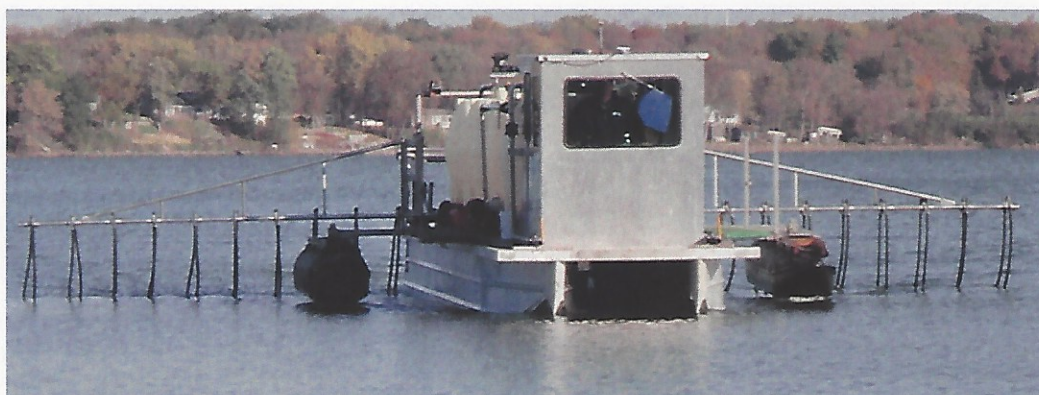
HAB Aquatic Solutions, Inc., is shown dosing Spring Lake with Aluminum Sulfate.
