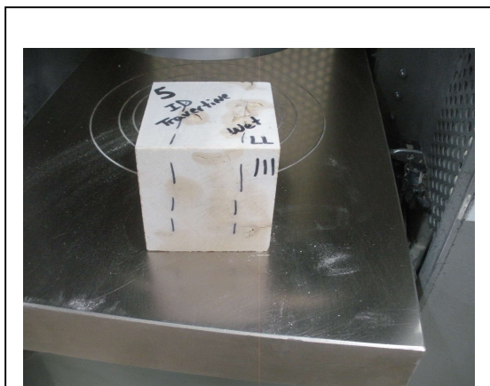
Photo No. 3 ASTM C170 – Pretest Condition Specimen
