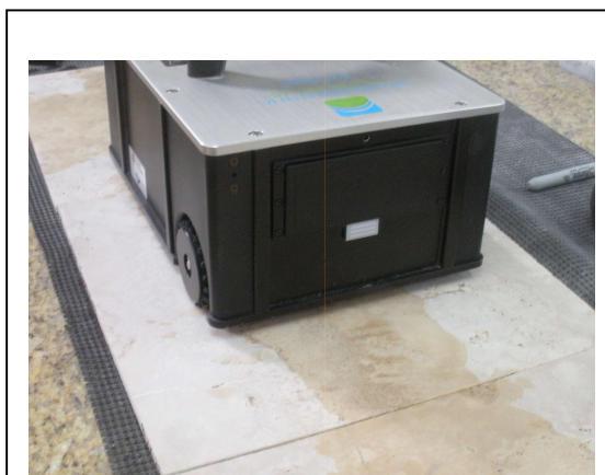
Photo No. 12 ANSI A326.3 – Test in Progress
