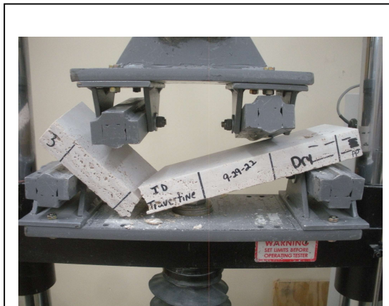
Photo No. 6 ASTM C880 – Representative Specimen Failure Mode
