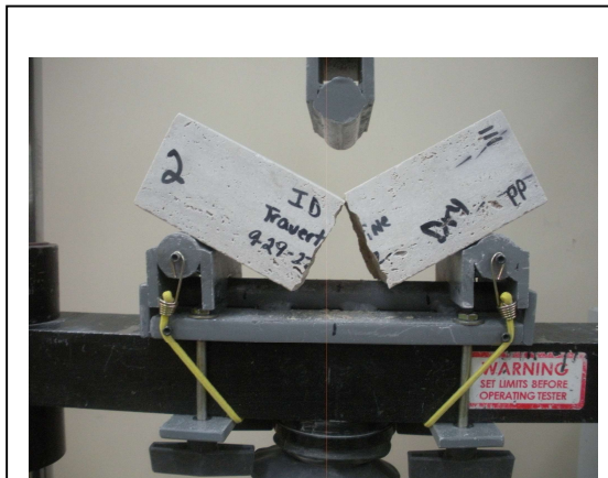
Photo No. 10 ASTM C99 – Representative Specimen Failure Mode
