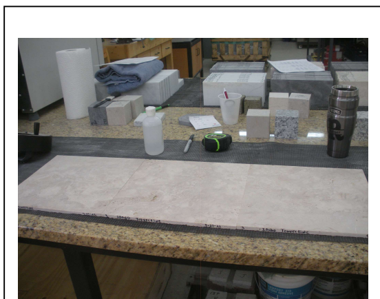
Photo No. 11 ANSI A326.3 – Test Setup
