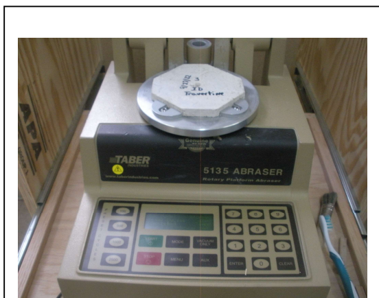
Photo No. 7 ASTM C1353 – Test Apparatus (Depicted with Pre-Abrasion Test Specimen)
