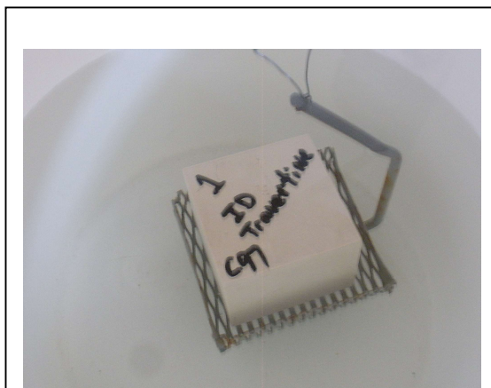
Photo No. 2 ASTM C97 – Suspended Mass Determination Depicted
