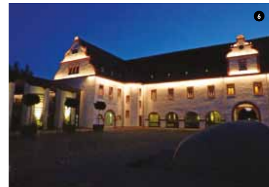
6 Heusenstamm Castle, Hesse, Germany After midnight, night mode starts automatically. Dimmable lights are set to 30% and switchable lighting turns off.
