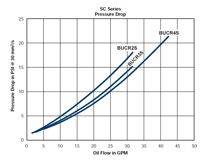
Pressure differential  $\Delta p$  depending on flow rate Q and the viscosity of the oil. Graph uses oil viscosity of 150 SSU. For oil viscosities other than 150 SSU, in the graph above multiply the  $\Delta p$  by the factor k for the corrected pressure drop.
