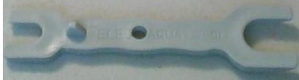
John Guest Fitting Wrench (Used to push down lock ring of fitting to remove tubing for plug)
