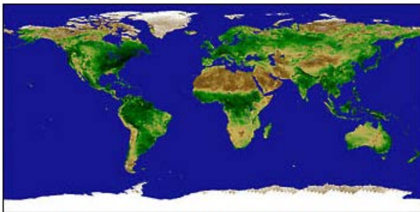
Normalized Differential Vegetation Index, Sept. 21–31, 1992 This is one of the simplest types of land cover classification maps, showing only the amount of green vegetation. Heavily vegetated areas are dark green, moderate vegetation is light green, sand, rock, snow, and ice are shown as tan and white.
