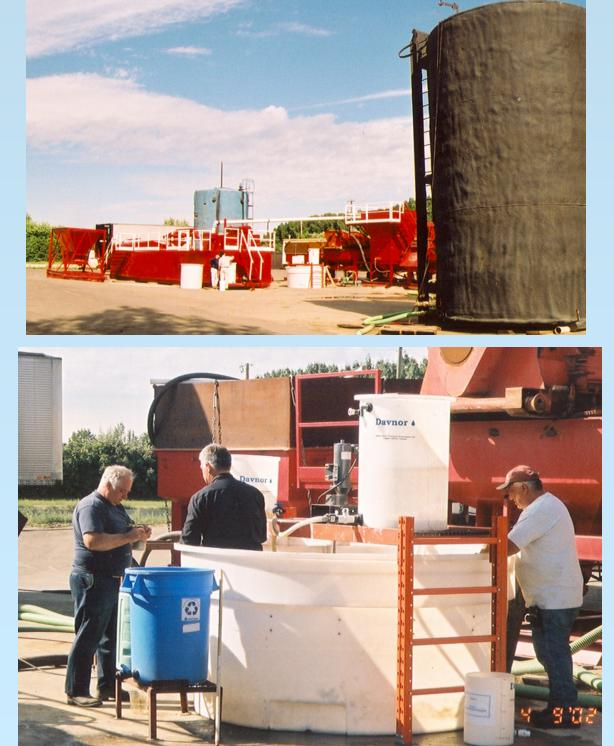
**Setting Up Field Test Reactors for 4 Cubic Meter Tests** on Flowback Water in Brooks, Alberta
