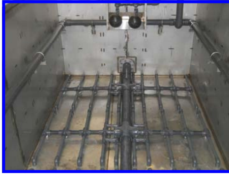
MEL Filter - 2m x 4m x 2m stainless steel body.
