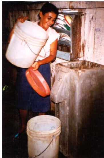
Concrete BioSand Water Filter being used in Nicaragua.
