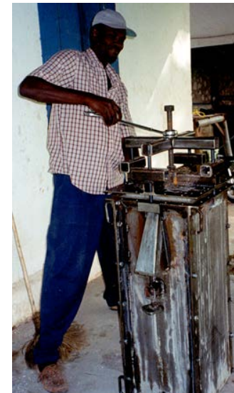
Concrete BioSand Water Filter being manufactured in Haiti.
