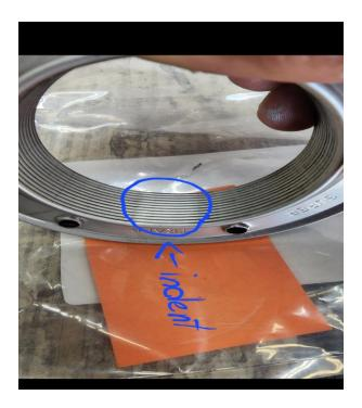
Pictures above show the indent on the inside of the disk by the supertrapp lettering.
