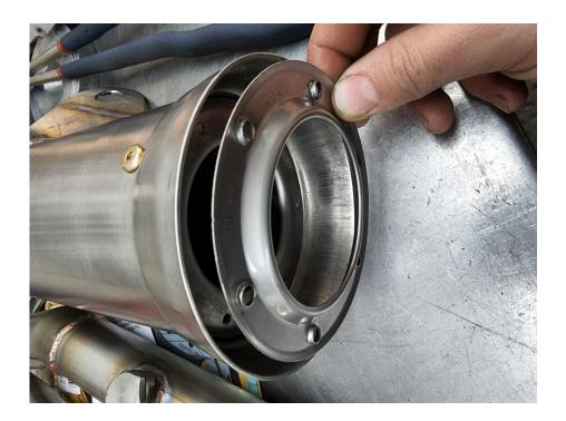
**Use high temperature anti-seize** on the bolts and cover all the threads with the anti-seize. **Torque bolts** to **15in-lbs**. Tighten in **criss cross pattern** a little bit at a time to tighten evenly.
