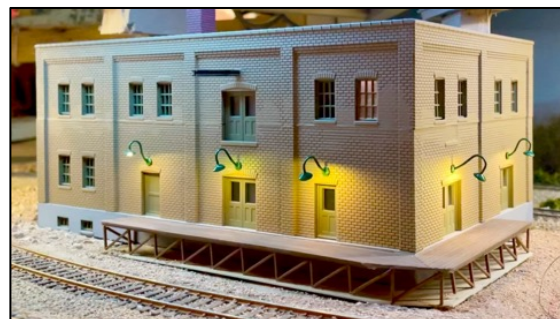
The first test building for John Mick's Arduino controlled lighting system. The system will cycle through a 24-hour day in twenty minutes. Individual lights can be programmed to cycles on and off throughout the day.
