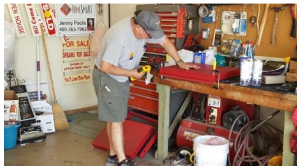
Bob Bridges roughs up paint on drawers in preparation for refinishing.
