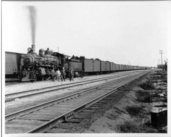
A lettuce train prepares to leave Phoenix in 1927. The refrigerated boxcars have ice shoved into their bunkers to keep the produce fresh.
