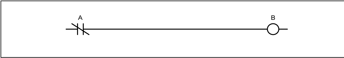
Figure 1-2 Normally Closed Logic
