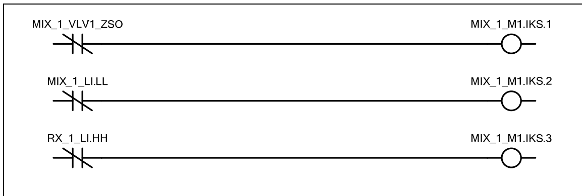
Figure 3-4 Discrete Motor Controller Interlocks
