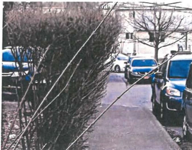
Photo 2.6.1-4 Hedge reducing useable width of sidewalk
